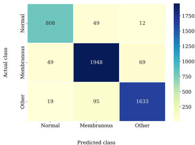
Figure 3. Wide-ResNet confusion matrix sum over the 10-fold cross-validation with a heatmap visualization.
